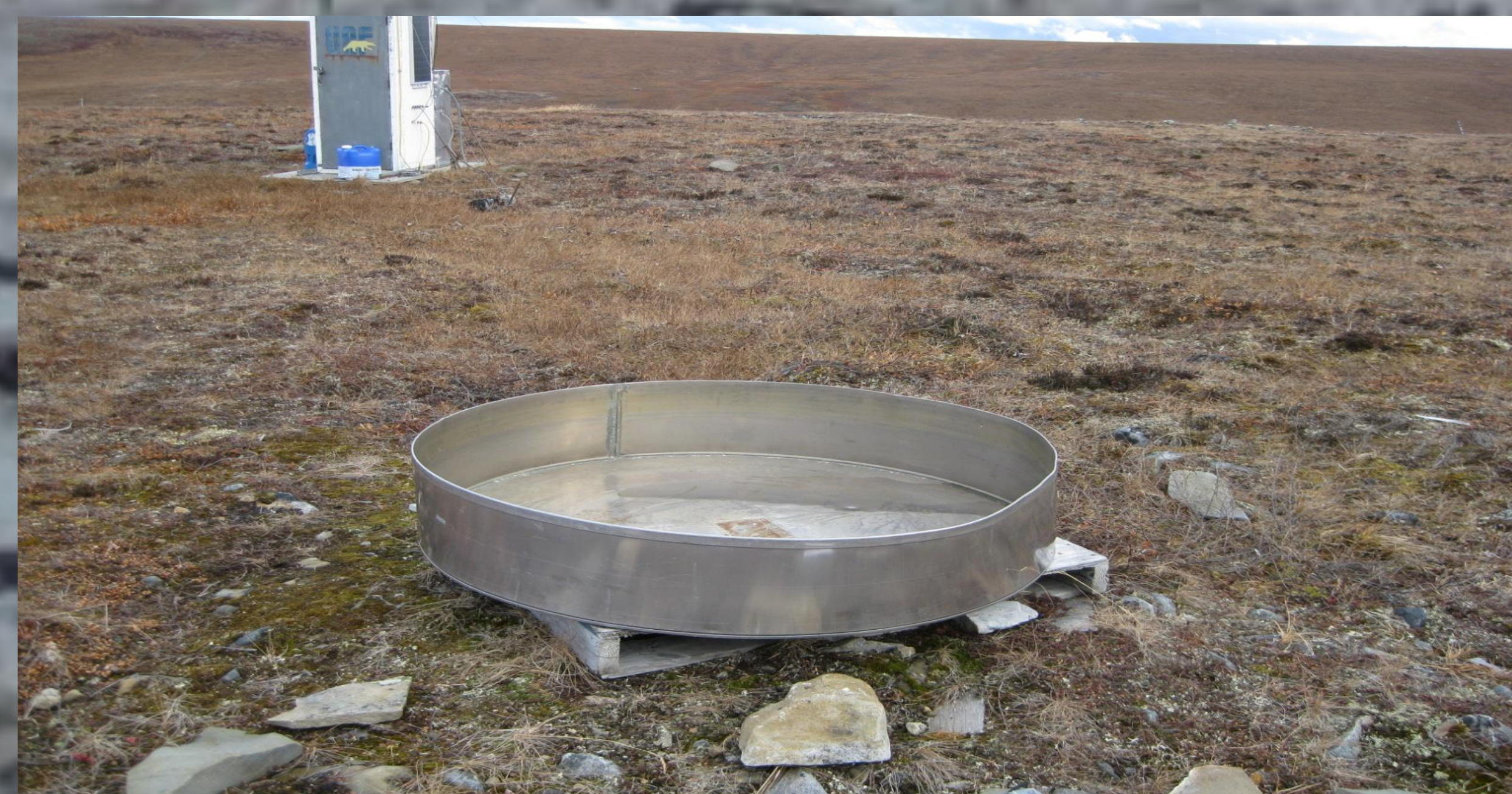
Figure 2- Evaporation Pan (standard Class A pan) located at the B site of Innavaik Creek Basin, North Slope of Alaska.
